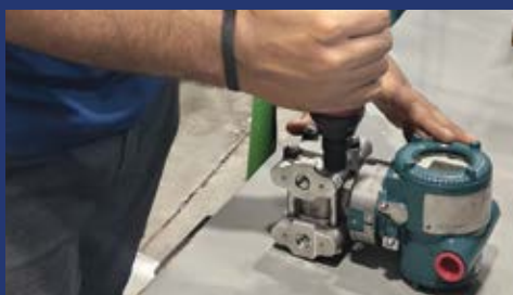
Reduced process time by 70% through power wrench implementation for transmitter opening process
