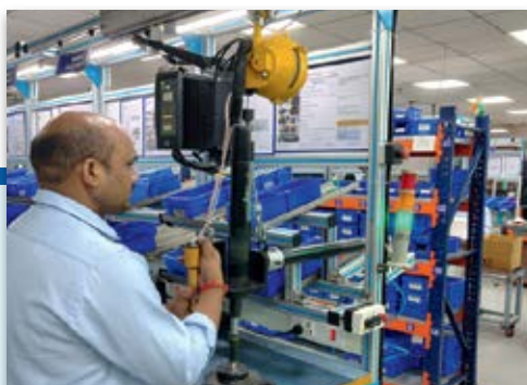
DC Nutrunner implemented for better torque control
