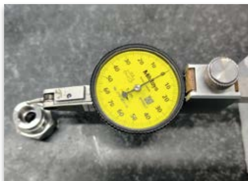
Bonnet face flatness identified as CTQ parameter and measured using micro dial gauge
