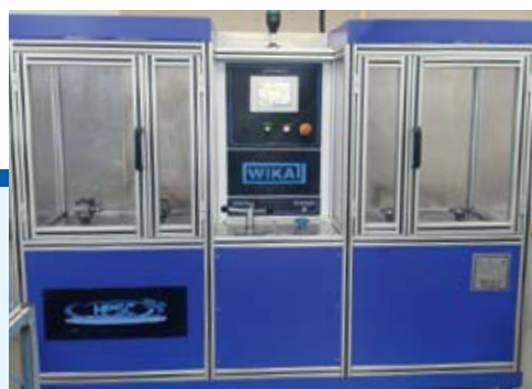
WII hydrotest bench for process standardization
