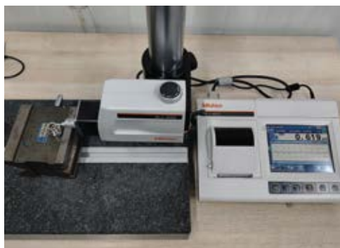
Upgradation in measurement to check Ra value of bonnet face
